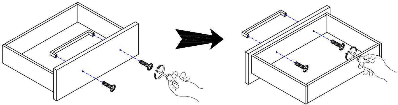
Take out handle from drawer, use screwdriver removing the bolts.
